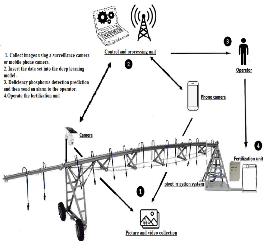
Figure 2. Shows the proposed idea of the Phosphorus Deficiency Detection System (PDDS).
