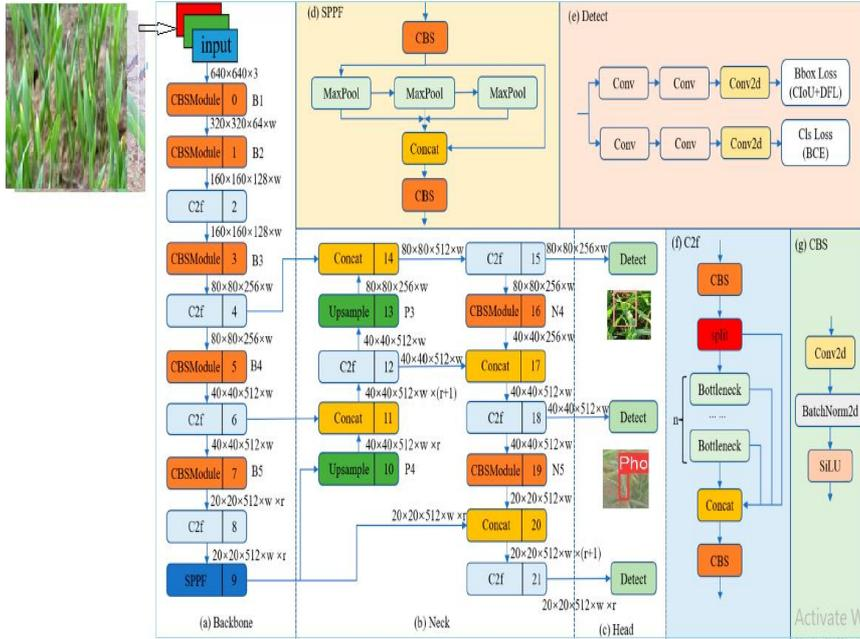
Figure 1. Architecture diagram for YOLOv8, adapted from (Wang et al., 2023).
